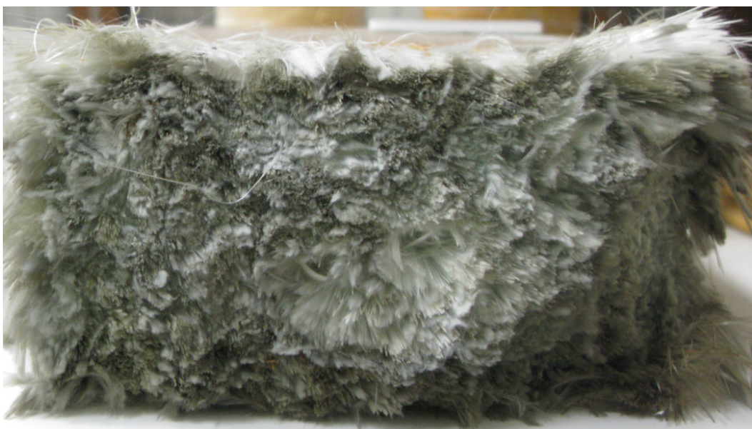
50 percent by volume ratio of glass fibres in the cross section of the FFU railway sleeper.
