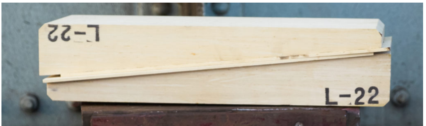
London Underground Chiswick Park, FFU wedge and layer pads.
