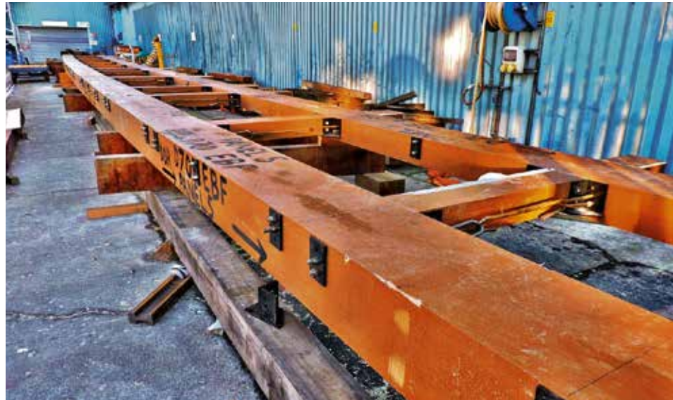
The prefabricated longitudinal bearer frames, manufactured from Sekisui FFU.
